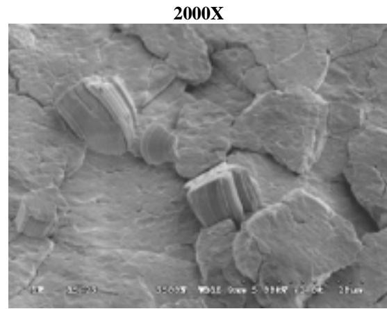
Figure 10. 2: SEM after 1000 TC of NEMI Condition on Pb-free Non-Annealed parts
