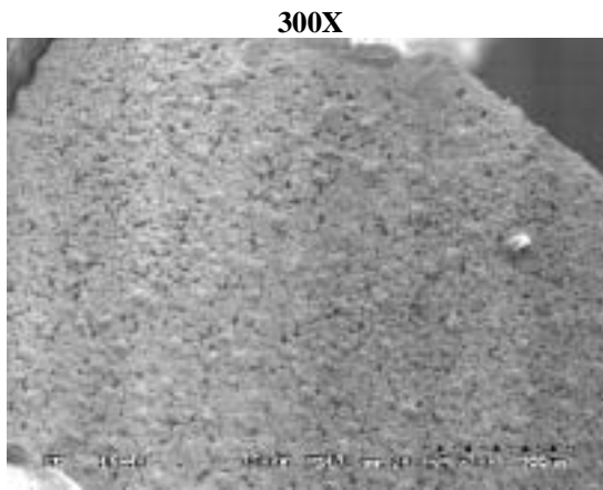
Figure 11: SEM after 1000 TC of NEMI Condition on SnPb Non-Annealed parts
