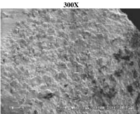
Figure 10. 2: SEM after 1000 TC of NEMI Condition on Pb-free Non-Annealed parts
